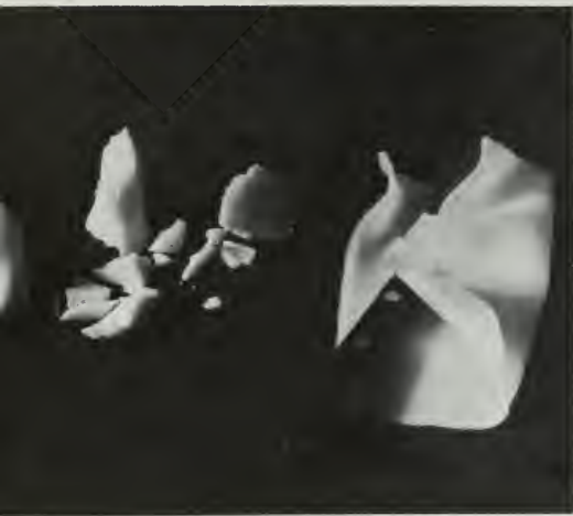
Sheet of an acetoglyceride folded over a spatula and (left) lumps of a completely hardened fat.
